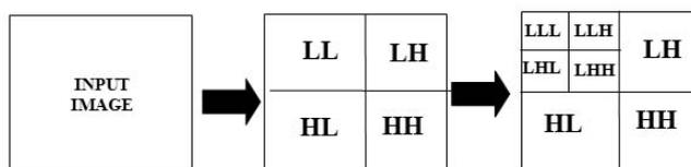
Figure 5. Analysis or decomposition hierarchy for 2-D DWT
