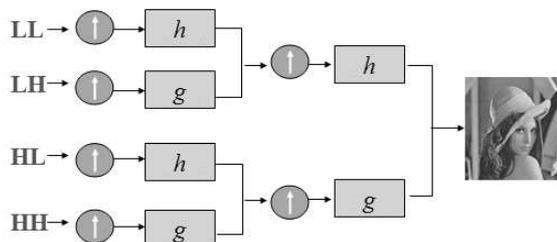
Figure 6. 2-D DWT synthesis or reconstruction tree
