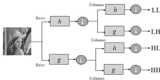
Figure 4. 2-D DWT decomposition or analysis tree
