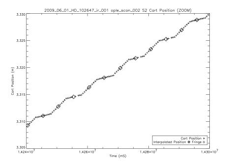
Figure 3.1: The position of the OPLE cart during a data set has a sloped saw-tooth pattern. This plot is zoomed in on a portion of the data set in order to clearly display the saw-tooth pattern. The diamond points indicate the location of the OPLE cart when a fringe was recorded.
