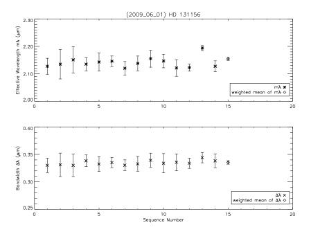
Figure 4.5: Results for HD 131156 OPLE cart data taken 2009\_06\_01. Top: Mean effective wavelength for each data set and the weighted mean value of those data sets (shown at the end of the sequence). Bottom: The width of the passband for each data set and the weighted mean value of those data sets.
