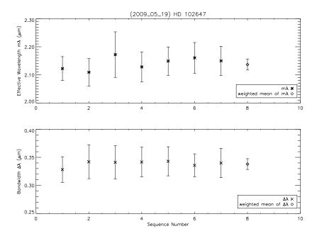
Figure 4.1: Results for HD 102647 OPLE cart data taken 2009\_05\_19. Top: Mean effective wavelength for each data set and the weighted mean value of those data sets (shown at the end of the sequence). Bottom: The width of the passband for each data set and the weighted mean value of those data sets.
