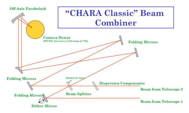
Figure 1.1: CHARA Classic beam combiner layout, showing the path of light through the system. (Figure courtesy of H. McAlister)
