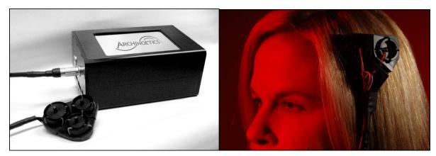
Figure 2. The OTIS fNIR device and sensor placement. Photo on left used with permission from (Nishimura et al., 2006). Photo on right taken by Stanley Leary and used with permission.
