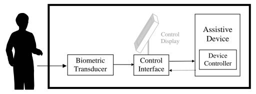
Figure 4. A model of a full biometric interface system. Adapted from (Mason & Birch, 2003; Mason et al., 2005).
