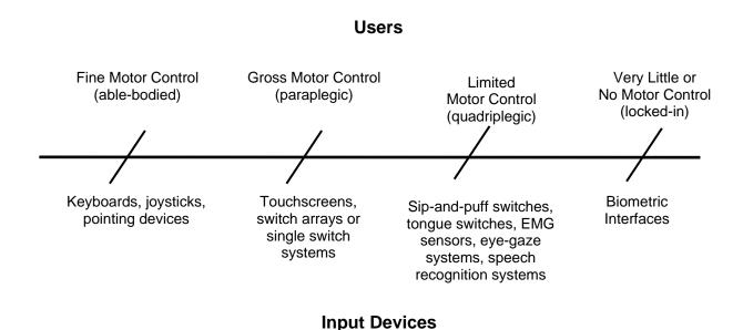
Figure 1. A continuum of disabilities and control interfaces. Figure adapted from (Moore, Storey, & Randolph, 2005).
