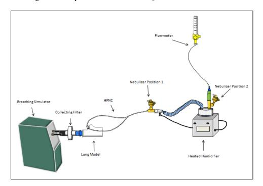
Figure 3. Experimintal set-up with HFNC.
