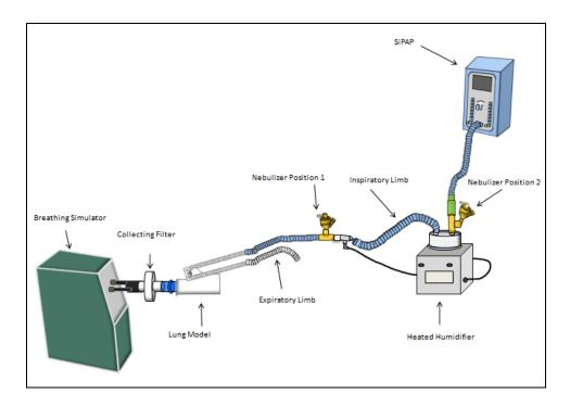
Figure 5.Experimental set-up with SiPAP.
