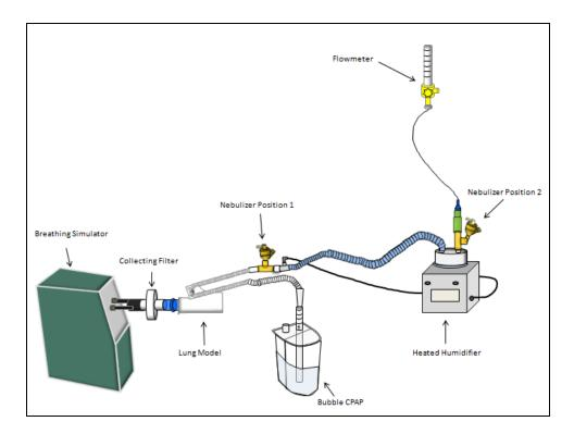
Figure 4. Experimental set-up with bubble NCPAP.
