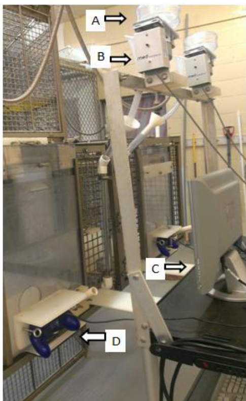
Figure 2. Diagram of the joint testing box (side view). Reward pellets sit in the reservoir (A) and are released by an automatic dispenser (B). Monkeys have a split-screen view on the computer screen (C) and control a cursor by moving a joystick on the controller (D) to touch moving targets.
