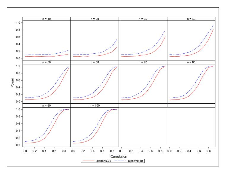
Figure 2.2 The power of 2D two-sample K-S test with T<sub>1</sub> statistics as a function of correlation by sample size and alpha level
