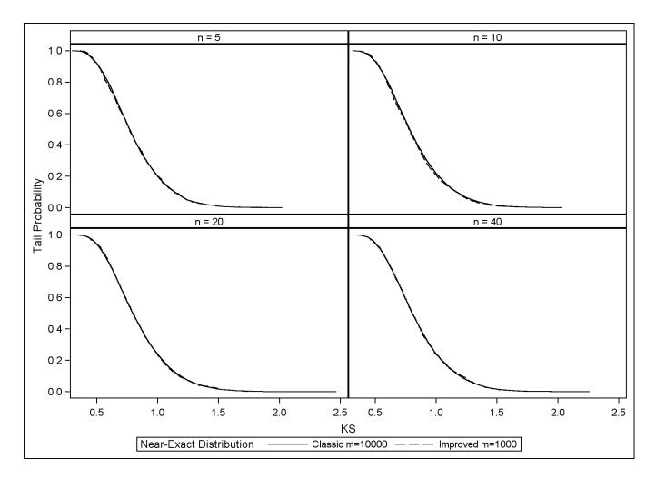
Figure 1.2 Tail probabilities of the classical and improved test statistics for one-sample K-S test (m= 1000 and k=1000)
