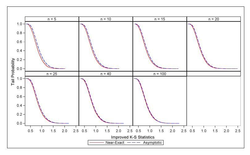
Figure 1.1 The near-exact and asymptotic tail probabilities of the modified 1D one-sample K-S test by sample size
