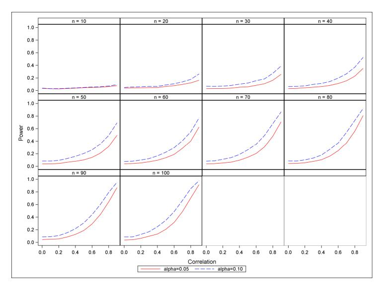
Figure 2.1 The power of the classical 2D two-sample K-S test as a function of correlation by sample size and alpha level
