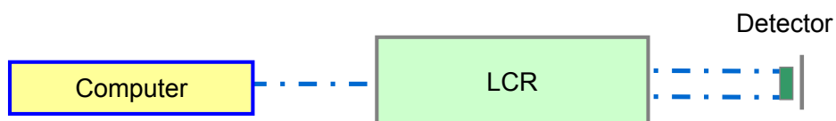
Figure 1.6: The computer-controlled Hewlett Packard 4284A LCR meter setup used to take C-V-f measurements of the dual-band detector structures.
