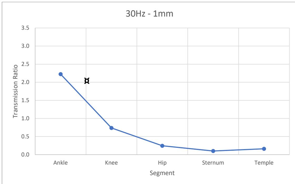
Figure 9: Transmission at each segment for the condition 30Hz and 1mm.
