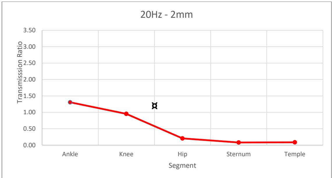
Figure 10: Transmission at each segment for the condition 20Hz and 2mm ( $\alpha$  denotes a frequency effect).
