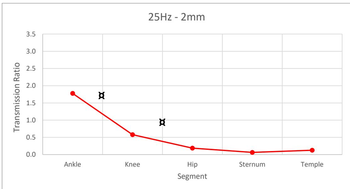
Figure 11: Transmission at each segment for the condition 25Hz and 2mm ( $\alpha$  denotes a frequency effect).
