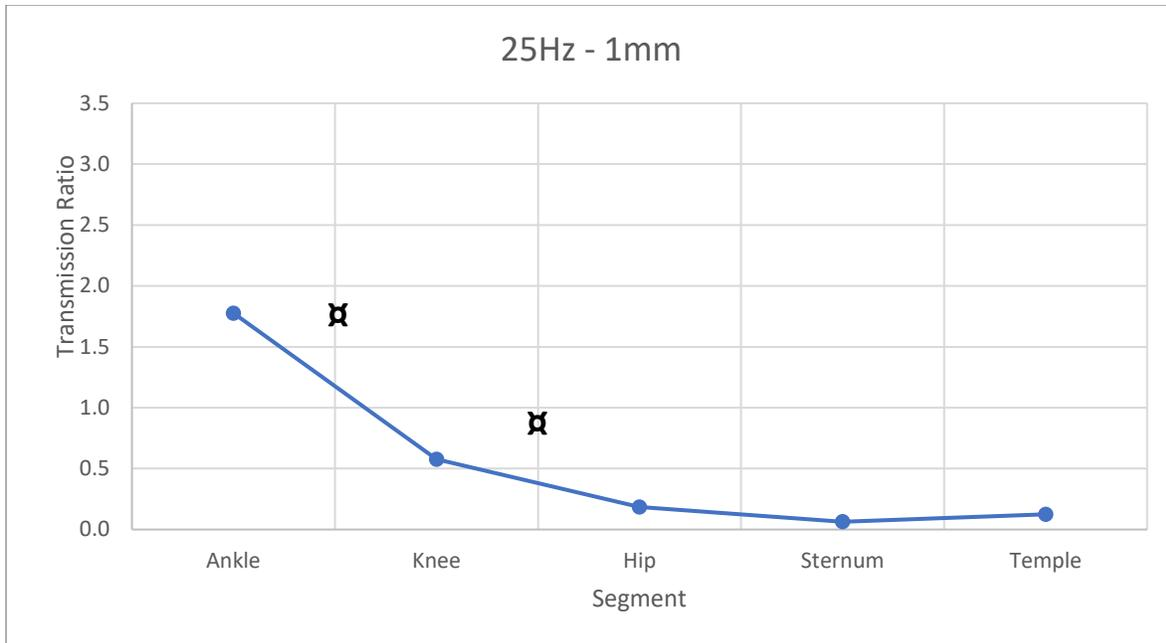
Figure 8: Transmission at each segment for the condition 25Hz and 1mm. (⌘ denotes a frequency effect).
