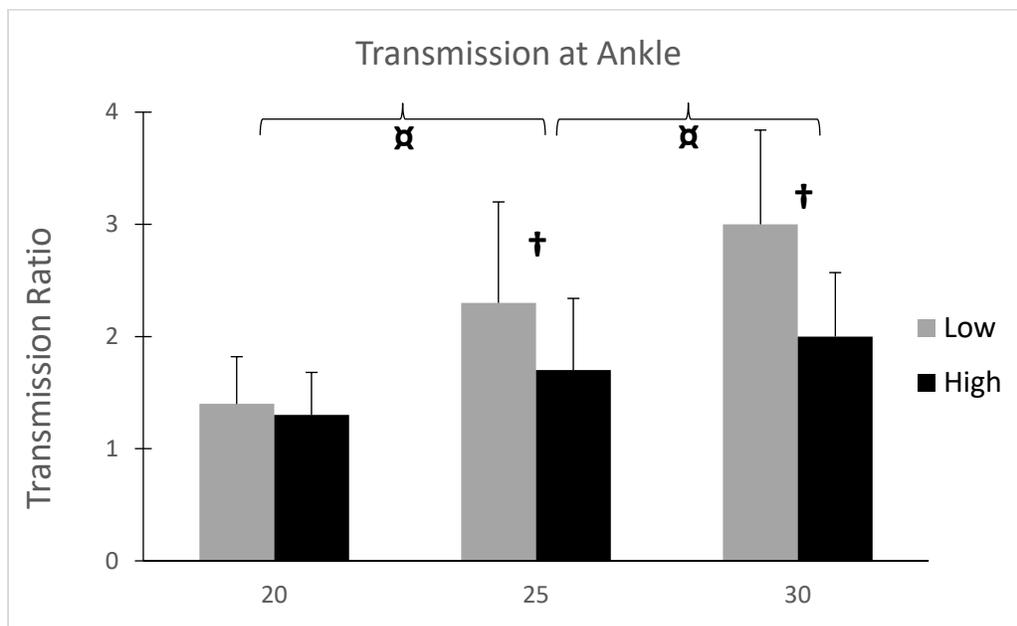
Figure 13: Acceleration transmission at the ankle (⌘ denotes a frequency effect and † denotes an amplitude effect)
