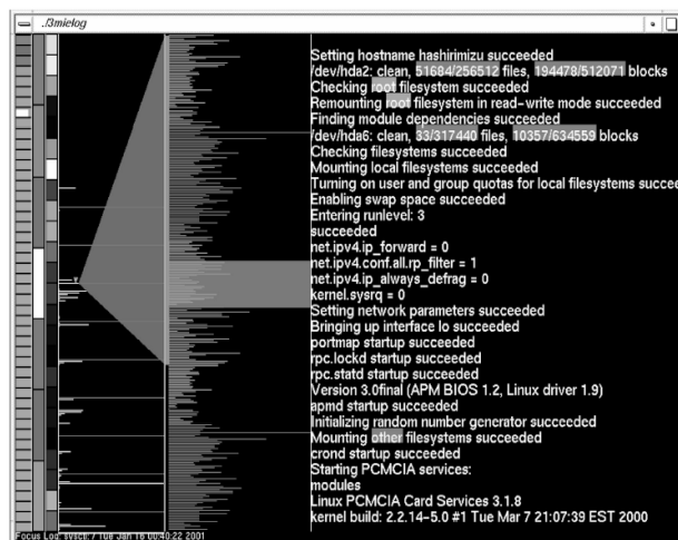
Figure 12. MieLog, [22], contains different visualization areas. The histogram is represented as horizontal lines. The lines vary in length. The zoomed in screen, located left of the message screen, shows the patterns generated by the histograms. Spikes can be easily observed, leading to the detection of anomalies.
