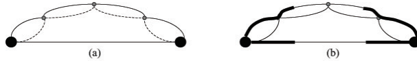
Figure 2.4. The Restarting Primal-Dual avoids the mistake of the Naive Primal-Dual. Part (a) shows duplication of the edges. Part (b) shows the components growing along the respective edges.
