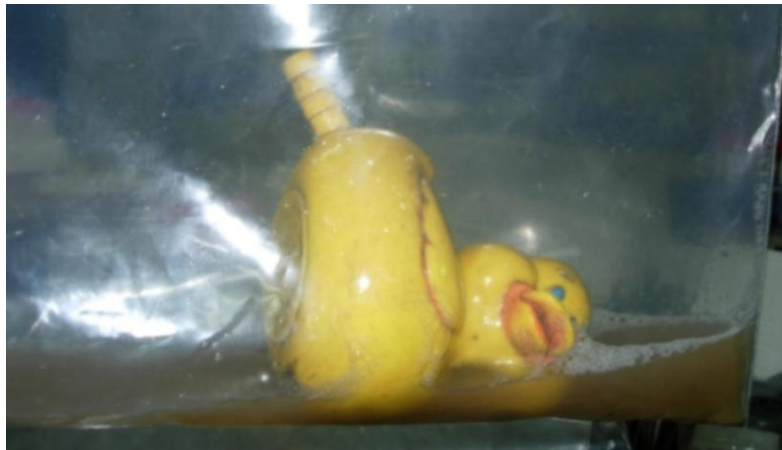
Figure 1: Example of sample collection bag with toy in wash solution.
