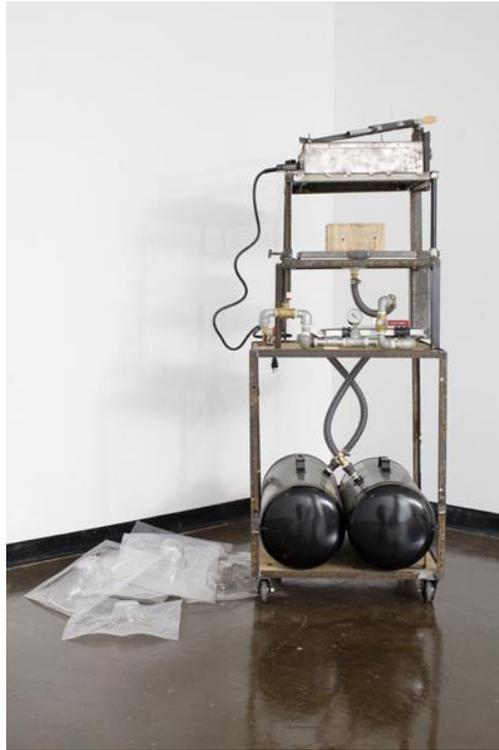
Figure 8. *Plastic Vacuum Forming Machine*
