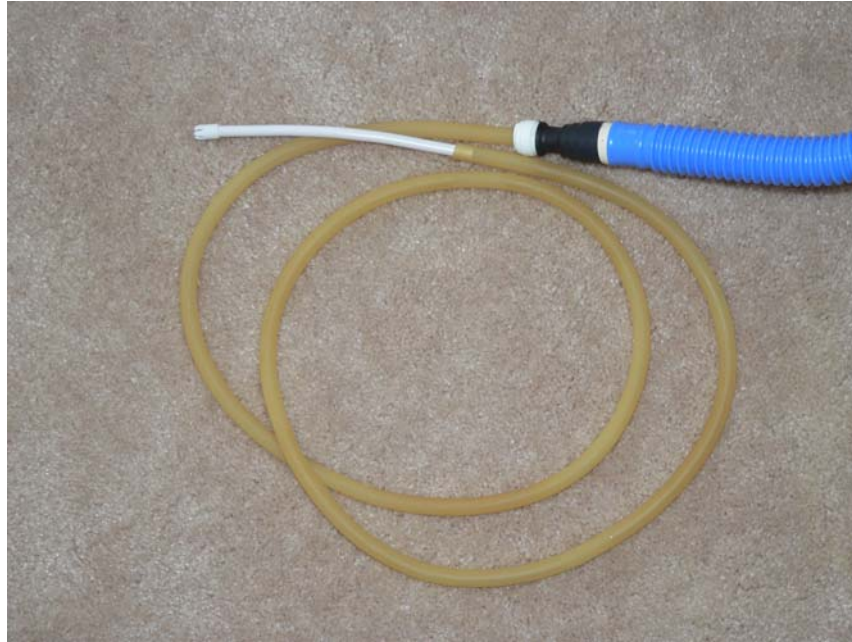
Fig. 4.8 Disposable silicon tube with mouth straw
