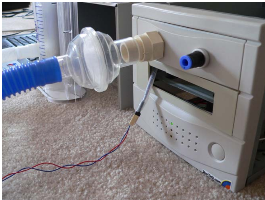
Fig. 4.7 Saliva trap biological filter (airflowmeter I/Os)
