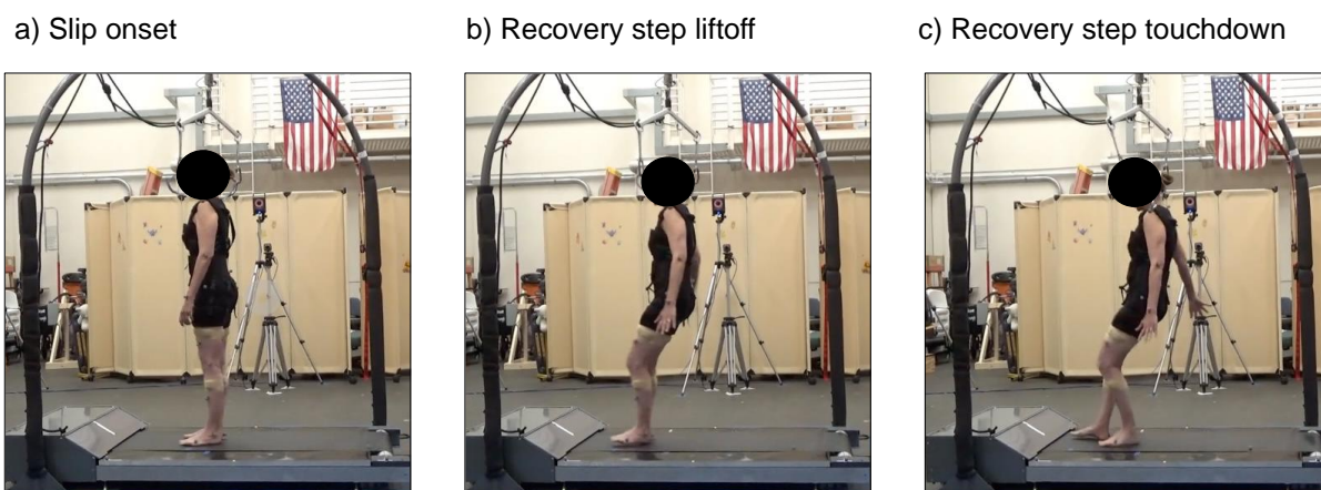
Figure 3.7 Images showing the three critical events of a) slip onset, b) recovery step liftoff, and c) recovery step touchdown during a standing-slip trial on the ActiveStep treadmill.
