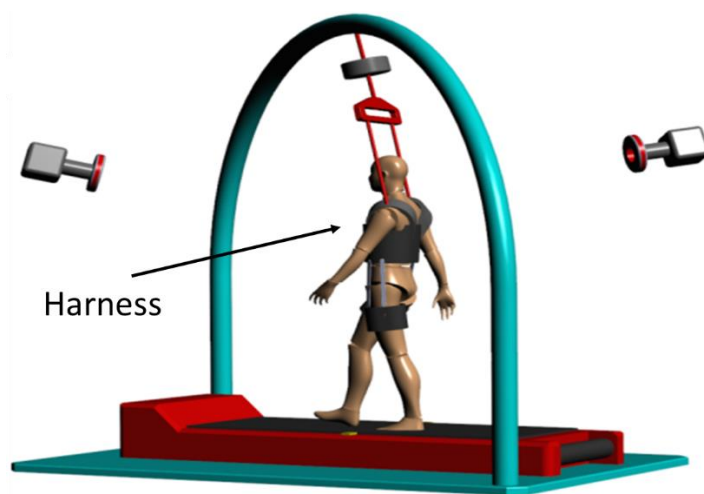
Figure 3.3 The ActiveStep treadmill used to deliver both the advanced and regular treadmill interventions. A full-body safety harness connected to an overhead arch via dynamic ropes
