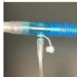
Figure 5 Auxiliary pressure sensor is attached between the fabricated airway and the TTL
