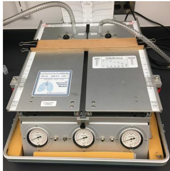
Figure 7 Dual Adult TTL with clamped board
