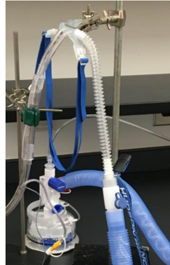
Figure 4 Hudson HFNC system with 22 mm corrugated tubing
