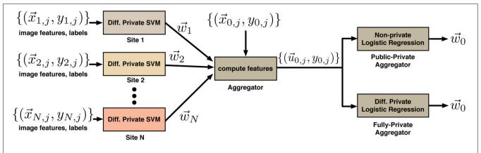
FIGURE 1 | System for differentially private classifier aggregation from many sites. The N sites each train a classifier on their local data to learn vectors  $\{\vec{w}_i\}$ . These are used by an aggregator to compute new features for
