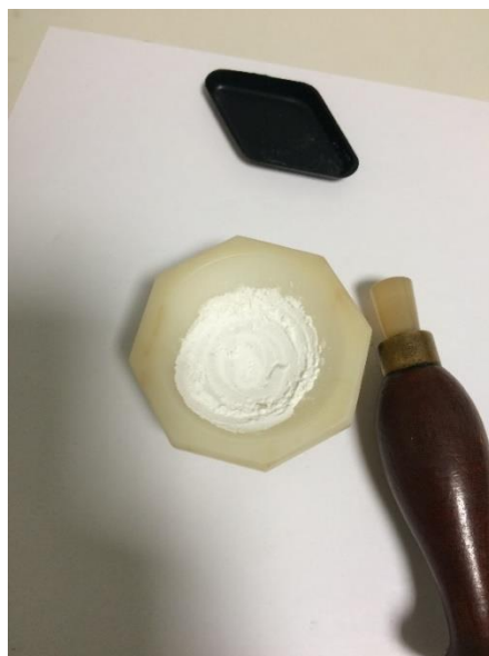
Figure 2.15 Sample and KBr after grinding with mortar and pestle
