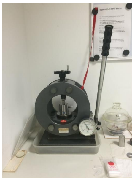
Figure 2.16 Ring press for pellets
