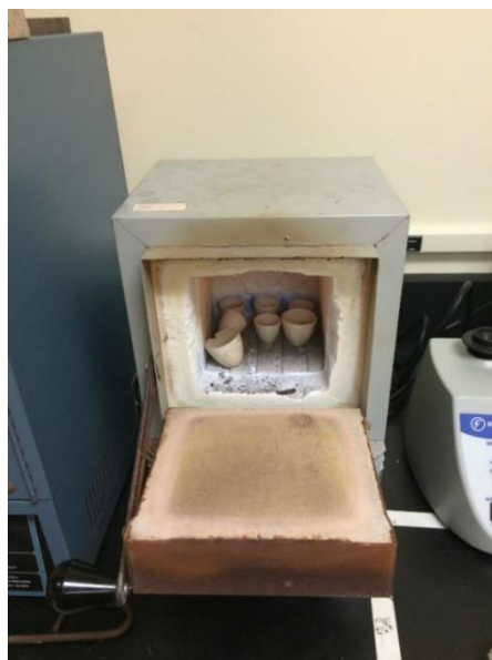
Figure 2.6 Thermolyne 6000 used for heating clay samples
