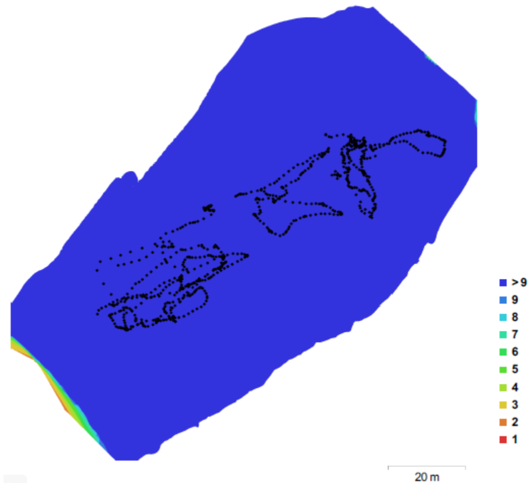
Figure 3.9: Locations where images were taken shown with image overlap statistics for SFPC
