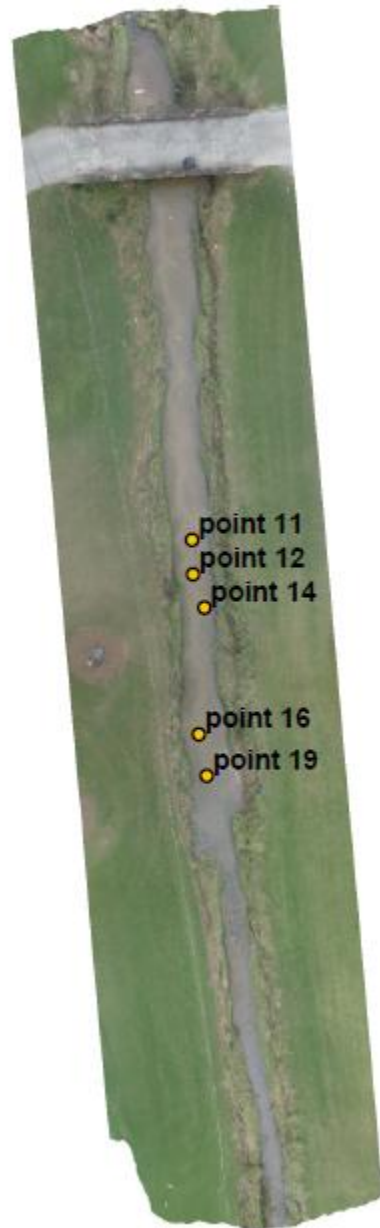
Figure 3.4: SfM model of the SFPC stream segment showing the locations of GCPs used as spatial reference
