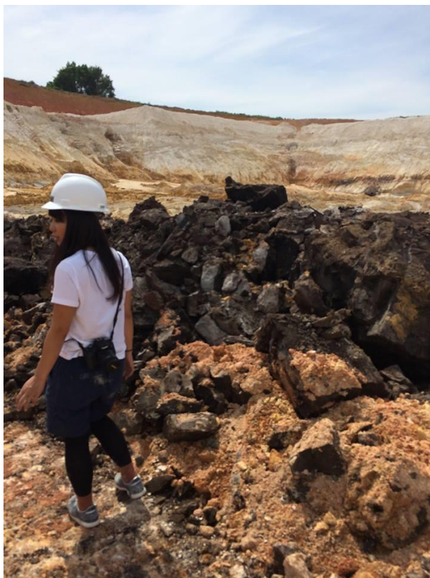
Figure 3: Dark colored Marion Member kaolins in foreground, lighter colored Jeffersonville Member kaolins can be seen in the background
