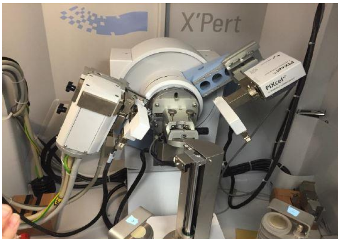
Figure 1. PANalytical XPERT-PRO XRD (Nikonova, 2015)
