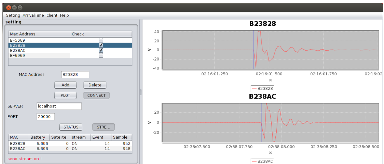
Figure 5.6 Stream data with arrival time picking on the monitoring and configuration tool.
