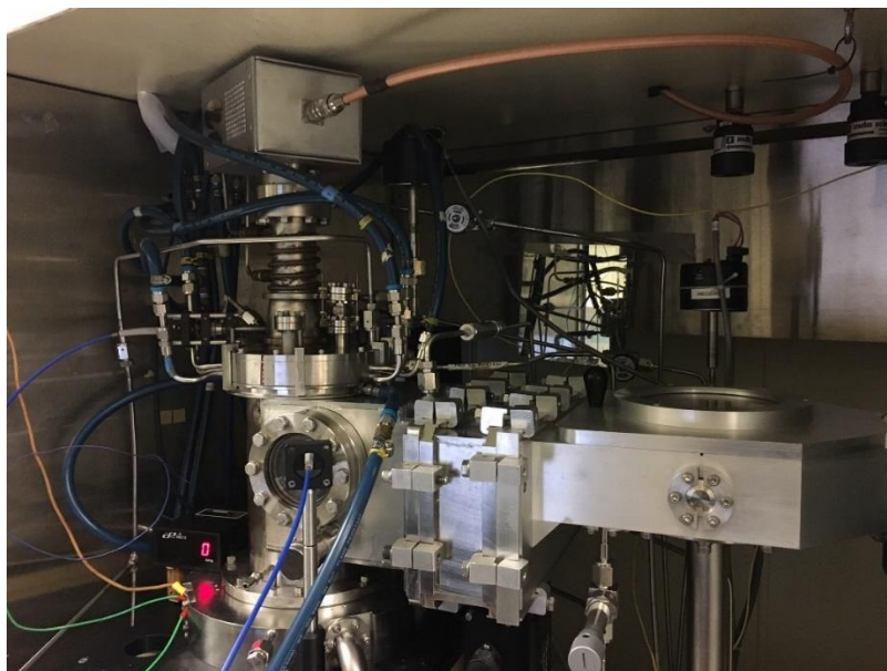
Figure 2-6 Picture of the MEPA-/PA-MOCVD reactor showing the plasma source on top and load-lock and gate valve on the right
