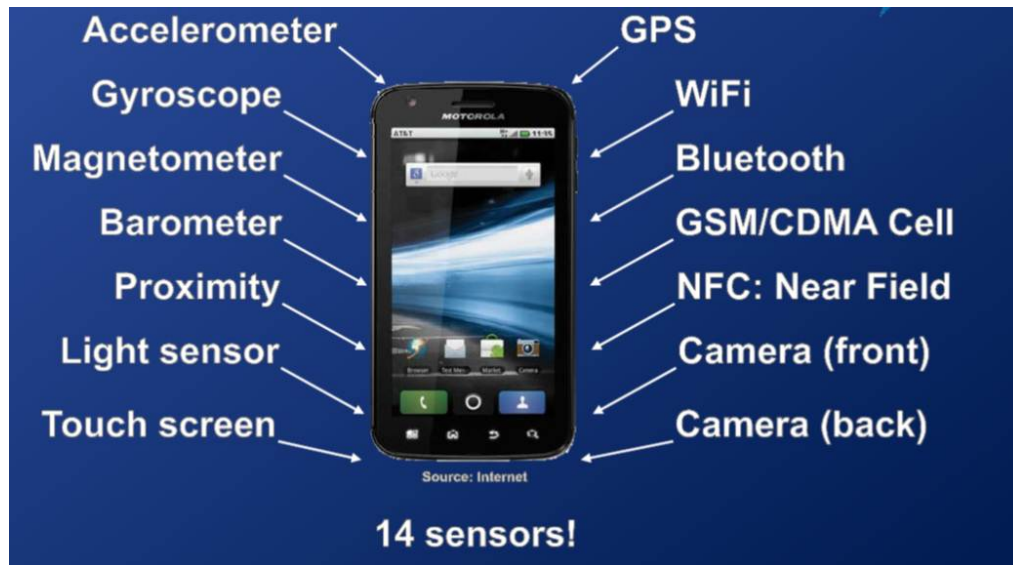
Figure 1.1. Sensors in smartphones
