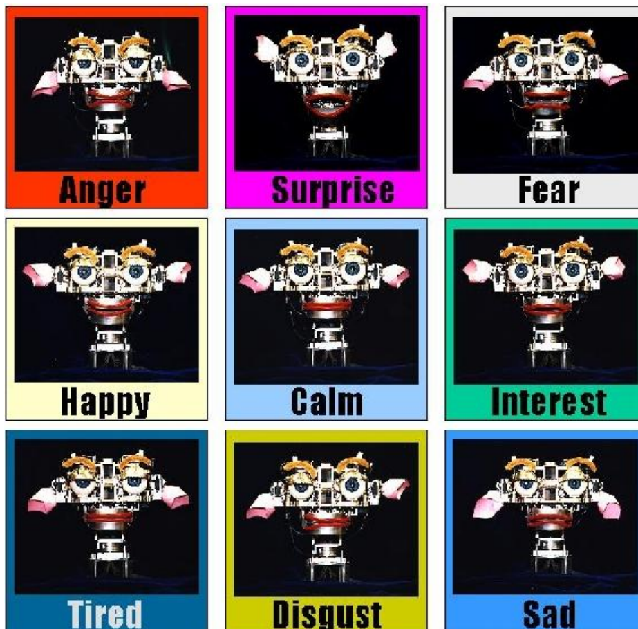
Figure 3.3. Kismet's facial expressions corresponding with recognizable emotions. By "Tired", Breazeal means Kismet is in an emotive state more commonly referred to as boredom. Reproduced from http://www.ai.mit.edu/projects/humanoid-robotics-group/kismet/kismet.html
