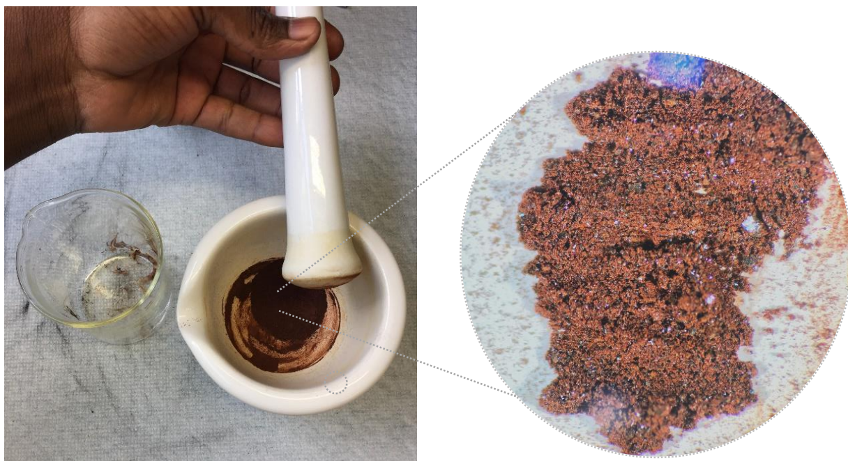
Figure 2-1 Synthesis of ferrihydrite. [A]. Mixing \text{Fe}(\text{NO}_3)_3 \cdot 9\text{H}_2\text{O}(\text{s}) and \text{NH}_4\text{HCO}_3(\text{s}) and [B]. Microscopic view of ferrihydrite.
