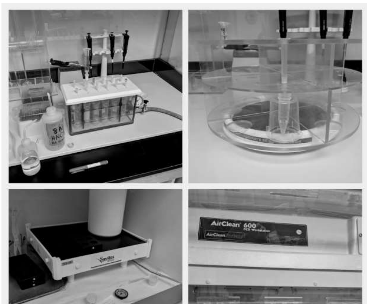
Figure 13 UGA's CAIS lab used for strontium and lead analysis. Top left – right: Strontium column set up. Lead column set up Bottom left – right : Savilex hotplate used to gelatinize samples. AirClean 600 – where the columns were setup.
