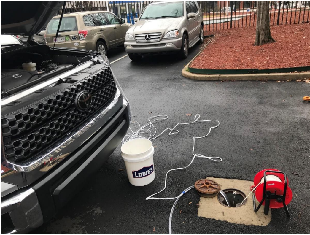
Figure 3.3 Pumping test (MW-01). The pumps were powered by (and connected to) the truck battery. The red piece of equipment is the water level indicator that was used to monitor drawdown and establish equilibrium conditions manually.
