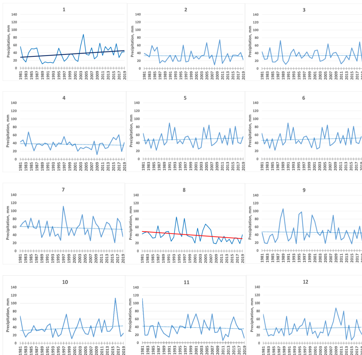
Figure 12. Region 1 mean monthly precipitation (adjusted) over 37 years (1981-2018). Month: 1-January, 2- February, 3-March, 4-April, 5-May, 6-June, 7- July, 8-August, 9-September, 10-October, 11-November, 12-December. Solid dark-blue line represents statistically significant increasing trend ( \alpha = 0.05 ; one-tailed). Solid red line represents statistically significant decreasing trend ( \alpha = 0.05 ; one-tailed). Dash blue lines represent non-significant trend.
