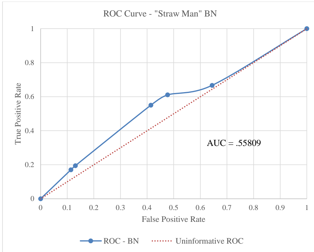
Figure 2.4. “Straw Man” BN ROC Curve. This figure illustrates the model’s predictive accuracy at different thresholds (solid line), as compared to an uninformative model (dashed line), as well as the AUC.
