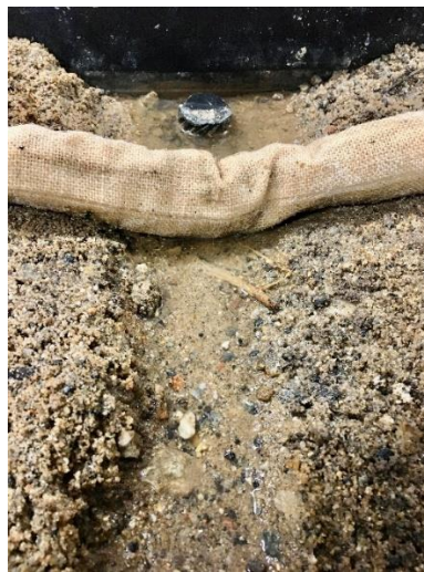
Figure 10 Trametes versicolor burlap mycofilter deployed in stream table.
