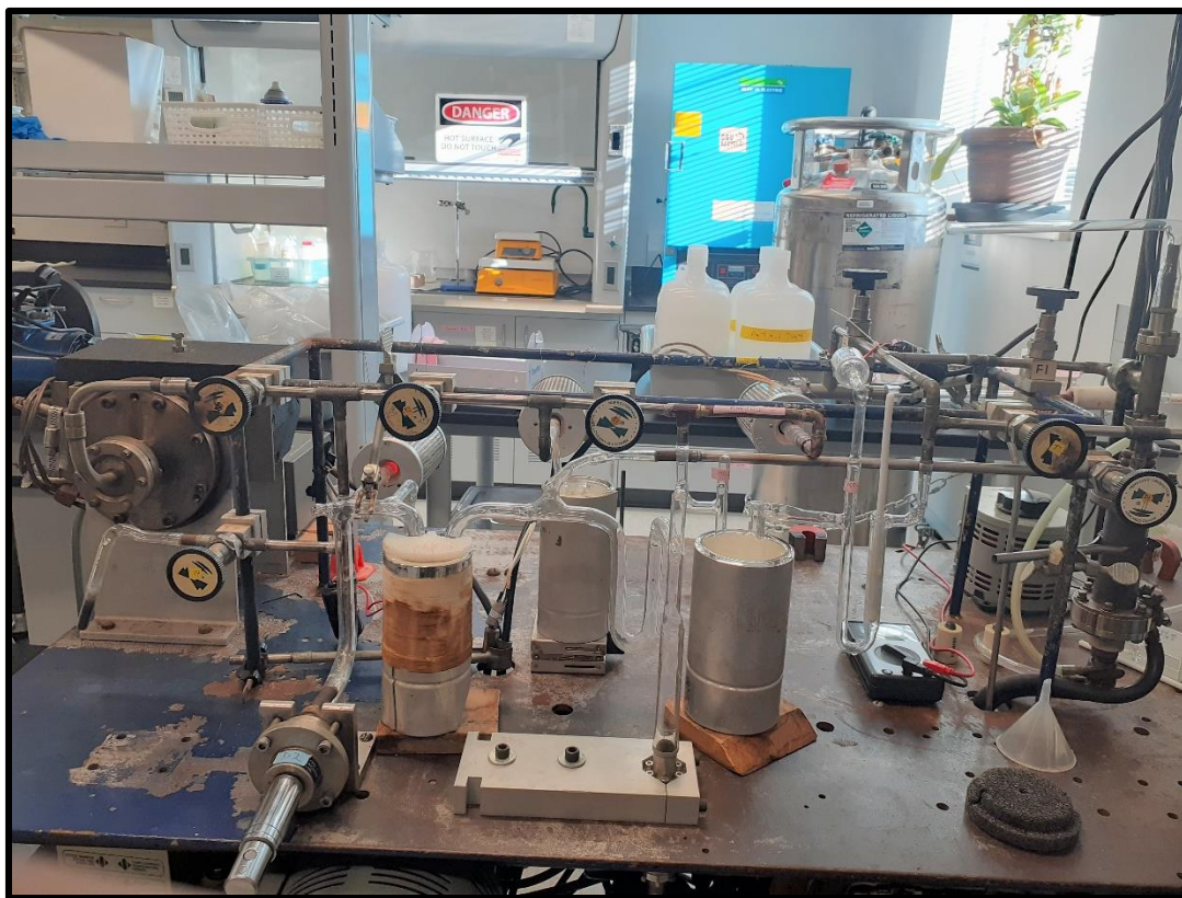
Figure 2-3 Photograph of argon extraction line showing the placement of the liquid nitrogen, used to trap condensable gases, and the MS 10 mass spectrometer (left).
