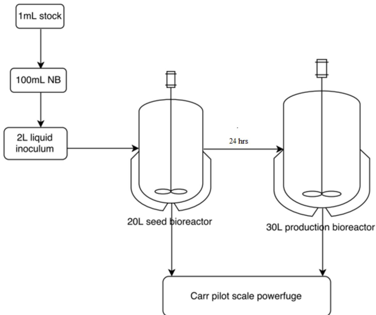
Figure 3.4 Production flowchart developed in this work
