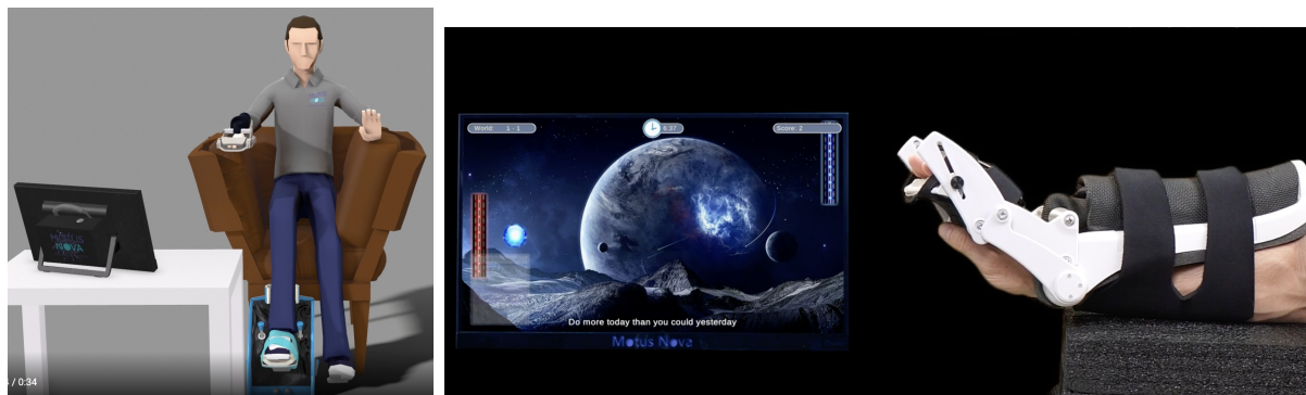
Figure 1.1: Patients do therapy sessions with the Motus Hand or Motus Foot using a pneumatically-driven exogenous robotic device that is worn on the affected hand/arm (depicted in the bottom panel). The peripheral acts as a game controller (through an angle sensor embedded in the wrist joint) that allows users to play therapeutic video games that are able to dynamically adapt to their needs and provide them the requisite assistance/resistance (computer screen in the bottom panel).
