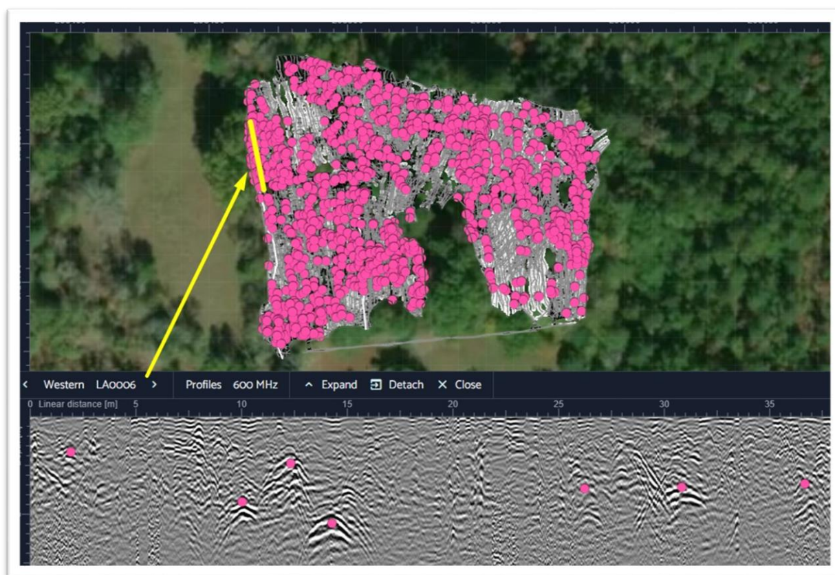
Figure 14: This image highlights the method for spatially plotting the locations of signatures interpreted as burials. I generated points at the tops of signatures featured on 2-Dimensional profiles. These points were spatially referenced automatically in Geolix GPR software.
