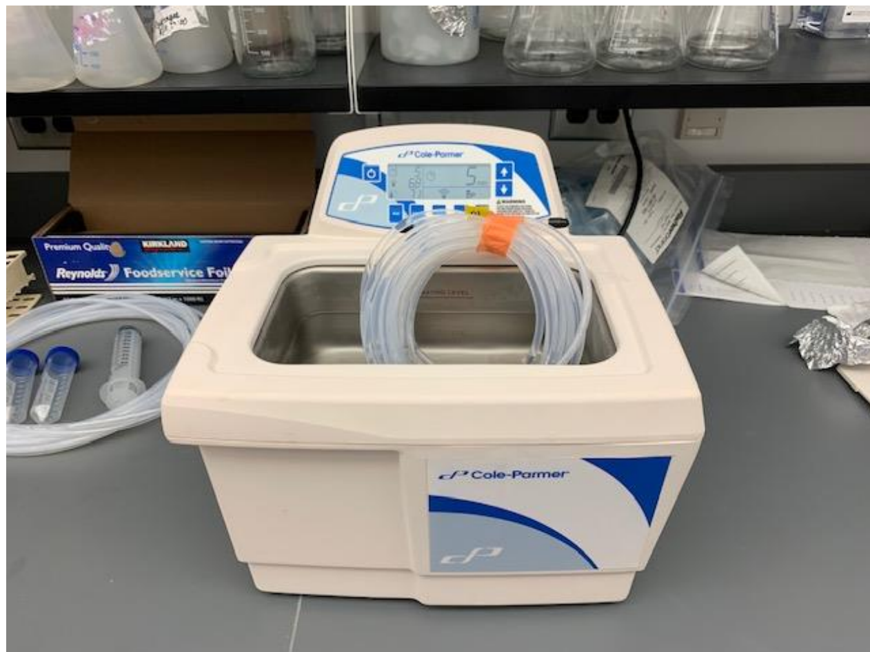
Figure 8. Sample Extraction Setup with Ultrasonic Bath Sonicator with FEP Tube
