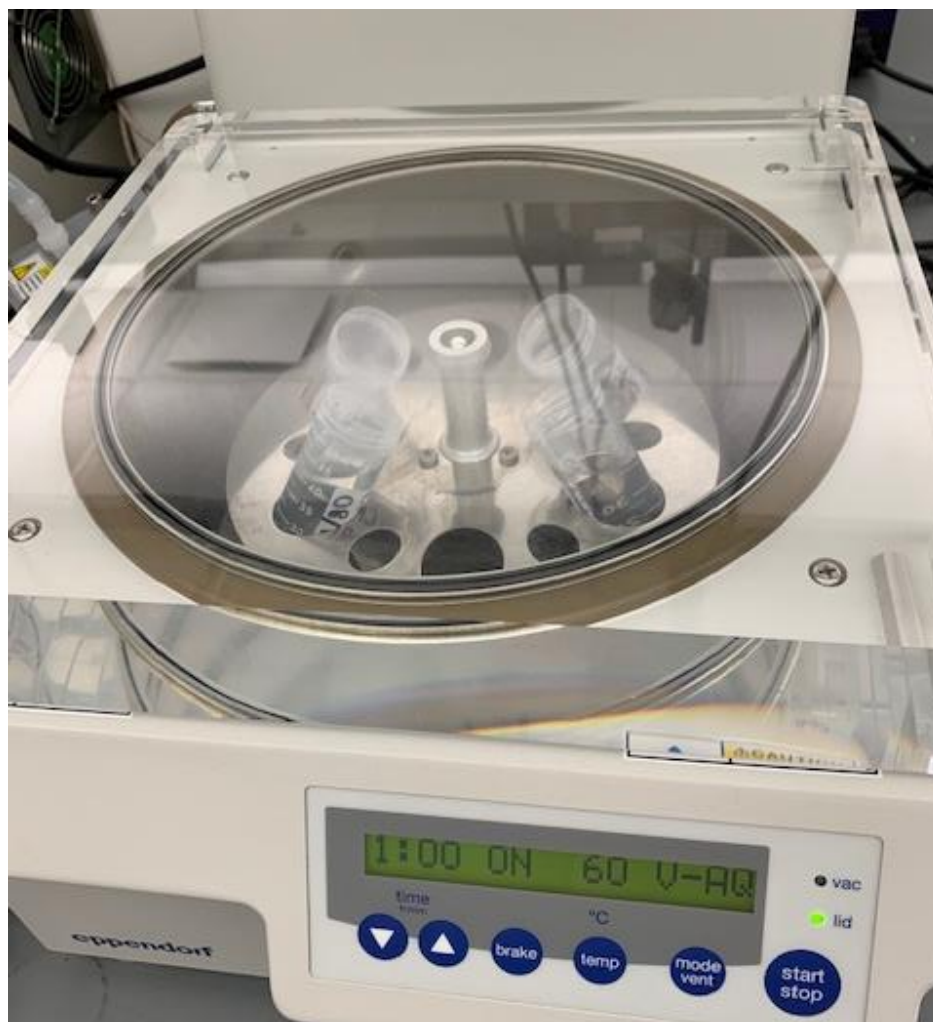
Figure 9. Vacufuge Process Setup After the FEP Tube Sample Extraction
