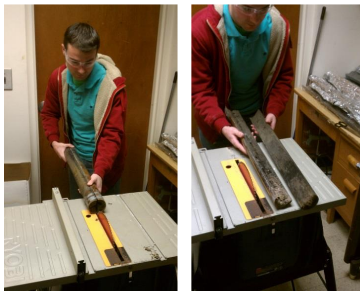
Figure 8. Splitting cores using a table saw.
