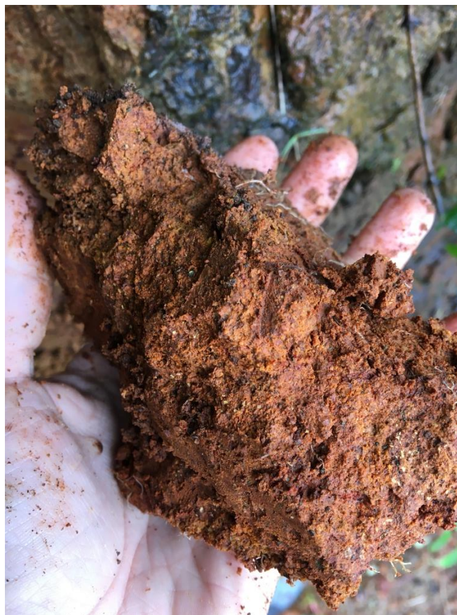
Figure 7: Heavily Weathered Tuff. The photo above is an example of a highly oxidized ash tuff. This deposit still slightly resembled an ash, as few grains were able to be distinguished. Although this tephra was able to be identified as an ash, some deposits are too oxidized to be identified.
