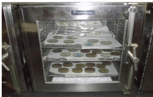
Figure 2.11. The desiccating cabinet containing the glass disks.
