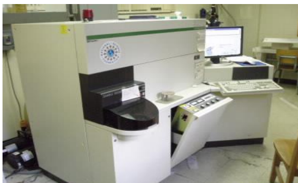
Figure 2.12. Rigaku 3270 X-ray fluorescence spectrometer at Georgia State University.
