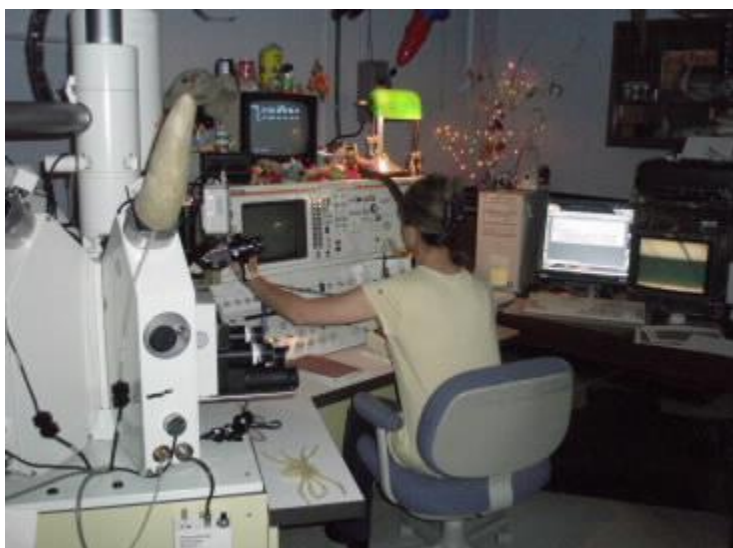
Figure 2.3. The EPMA lab at UGA. It includes, from left to right, an electron gun, and sample chamber with detector array, control console, and monitors.
