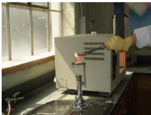
Figure 2.10. Pouring the melt into the hot mold.
