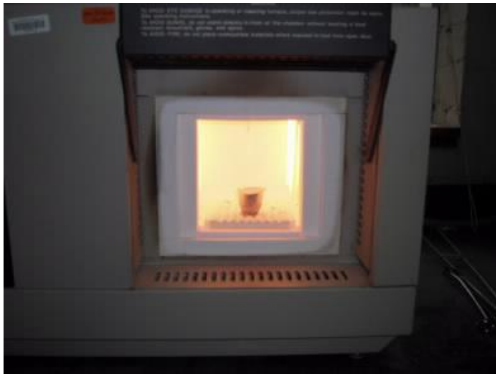
Figure 2.8. The platinum crucible containing the sample and flux in the 1100° C furnace.
