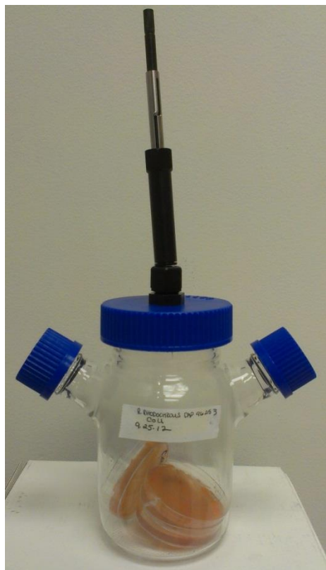
Figure 38: 250 mL Bellco (Vineland, NJ) Spinner Flask set-up used for SPME sampling.
