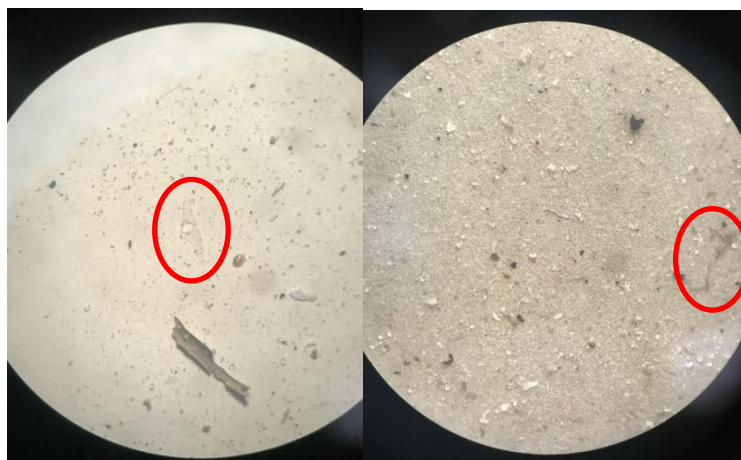
Picture 2. (Left to right) A clear plastic piece of microplastic extracted from sand sample N089A and a clear filament extracted from sand sample N041A.
