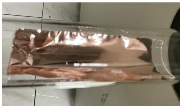
Figure 1.4 graphene on copper after 20 minutes LPCVD growth.
