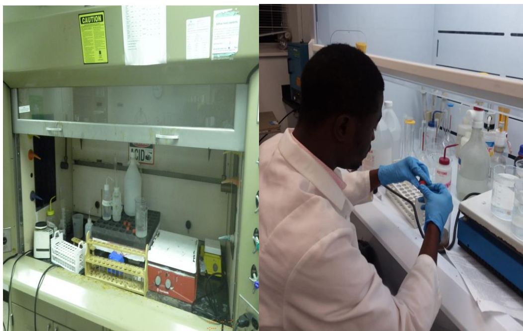
Figure 4: Figure Showing the fume hood used in acid treatment and acetolysis in the Lab.
