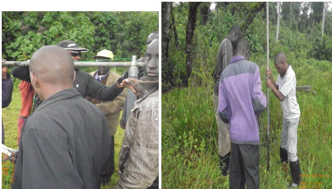
Figure 2: Field images showing the Modified Livingstone Corer used to recover sediment.
