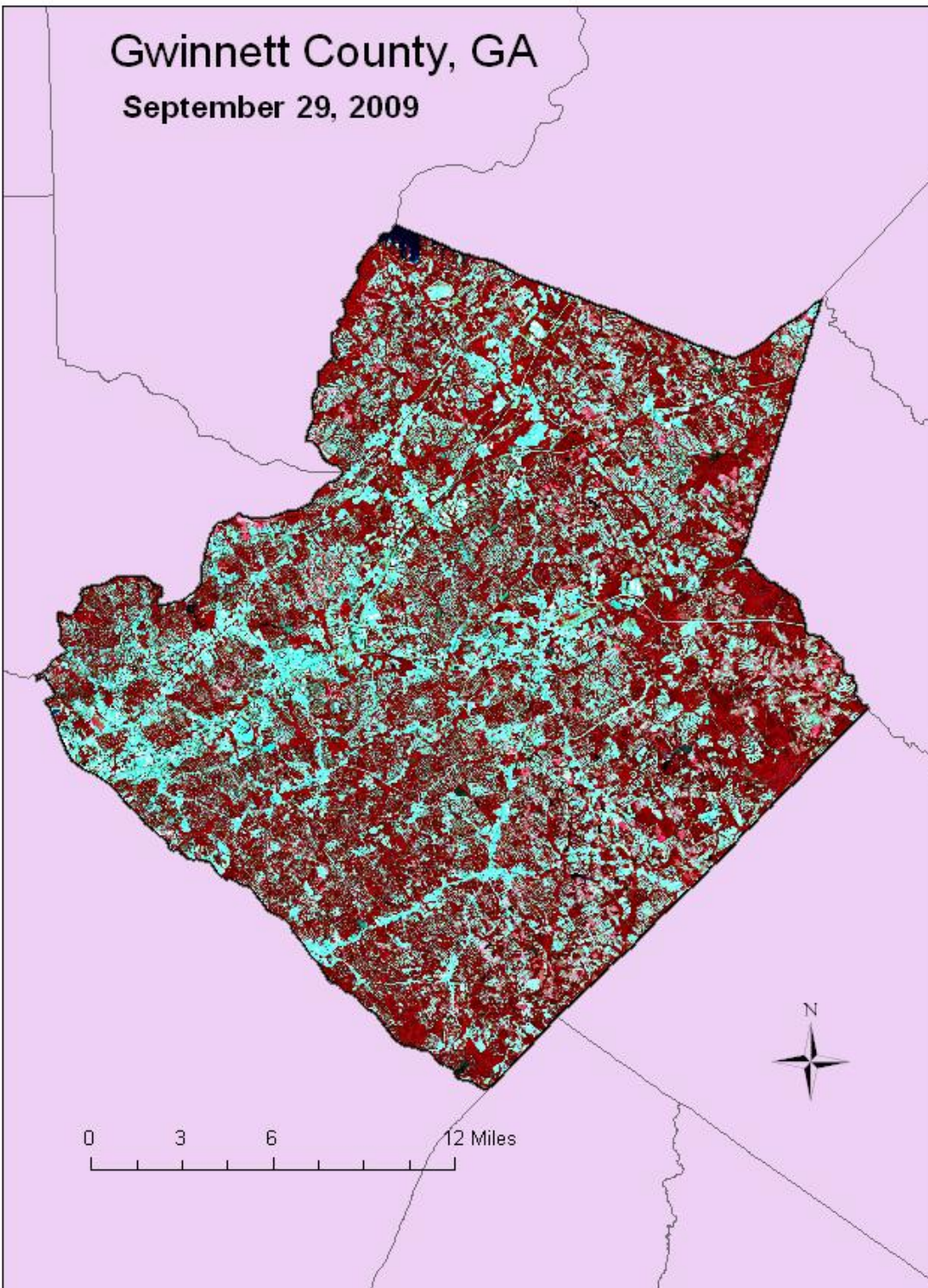
Figure 3. A map of Gwinnett County showing a false color Landsat Thematic Mapper image of the county taken on September 29, 2009 (bands 4, 3, and 2 displayed as red, green, and blue). Red in this image shows vegetation and the light blue areas are paved surfaces and buildings.
