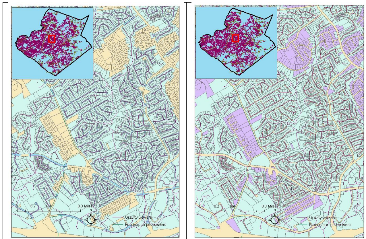
Figure 7. Close up view of a portion of Gwinnett County, Georgia showing the properties that overlap the 75 foot buffer around the sewer lines that would be the properties (in blue) serviced by the sewer system.
